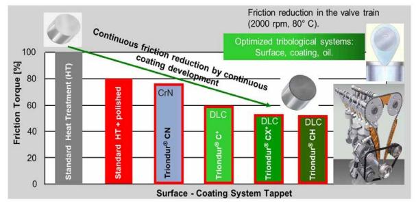
Figure 4: Measures reducing valve train friction (photo: SCHAEFFLER AG)
