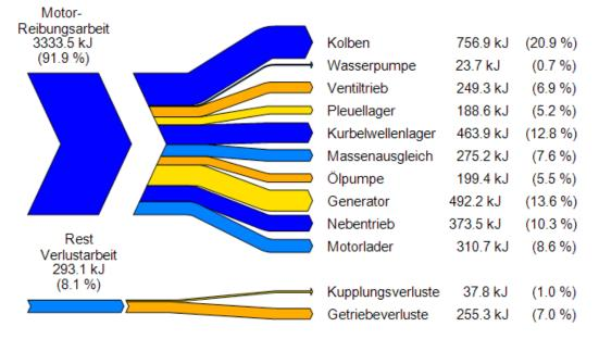
Figure 2: Friction broken-down to the various powertrain aggregates [14]
